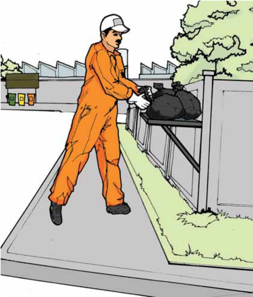
Figure 2-2: Waste collection work becomes much easier when waste is placed at waist level of collectors.
