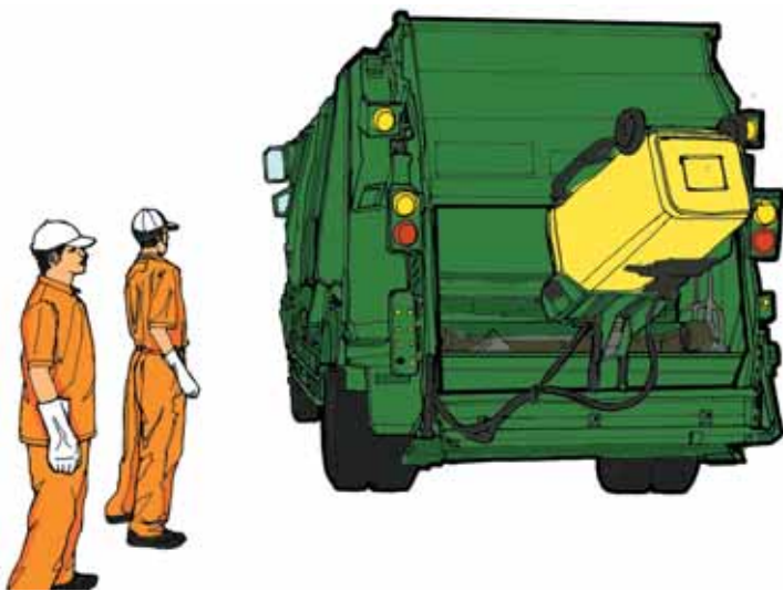
Figure 8-1: Stay away from rotating parts of the waste truck for safety. Use mechanical lifters if available.
