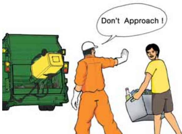
Figure 8-3: Don't allow members of the community to throw their waste directly into the hopper.
