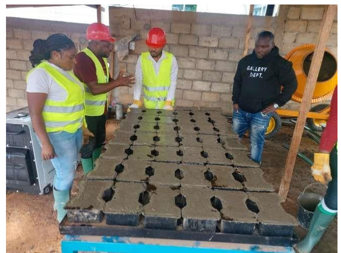
Photo: vibration of pavement molds, though the vibration has to be improved upon to carry full capacity as seen
